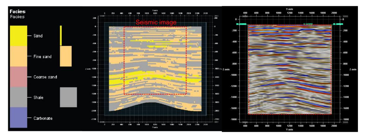
Realistic synthetic models: amplitude and frequency content also correspond to 'real' surveys Misinterpretation to include faults = epistemic uncertainty
