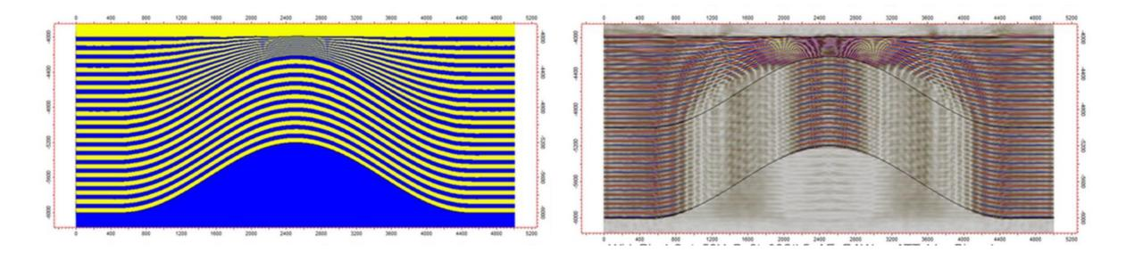
Lack of reflected energy due to illumination of the geometry
