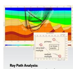
Improve your understanding of ray propagation in isotropic or anisotropic models. Identify and analyse primaries, multiples, and multiple ray paths using re-tracing functionality.
